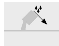
Flush difuser to minimise water and dust residue
